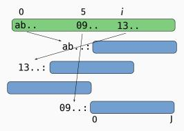
Example of a 2-D array implemented as an 1-D array of pointers to 1-D data arrays
