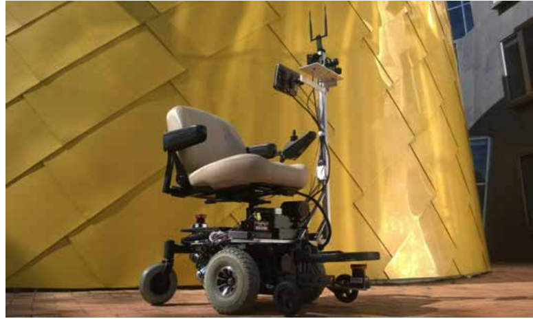
Figure 4: A robotic wheelchair that was used as the experimental platform for inferring maps and behaviors
