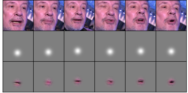
Fig. 4. Examples of mouth region masking during training, showing video frames (first row), 2D Gaussian masks (center row), and masked video frames (bottom row).
