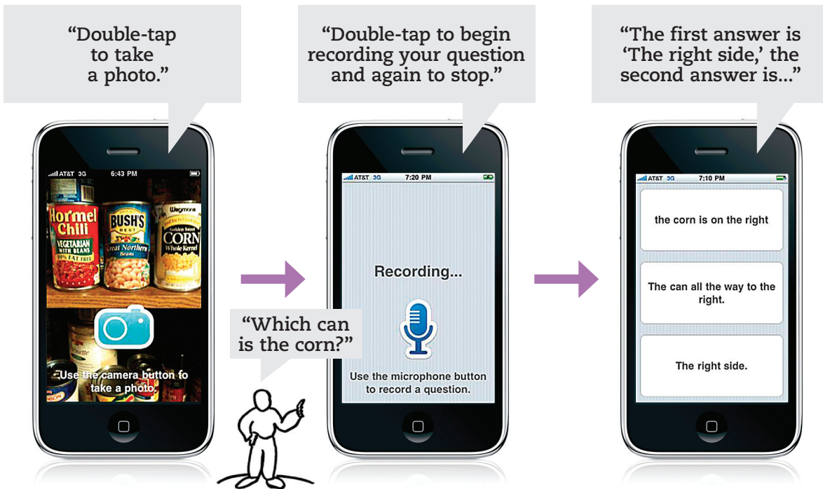
► Figure 1. VizWiz works in three steps: a blind user takes a picture and speaks a question, which are forwarded to the crowd for answering, and then answers are returned to the device from the crowd.
