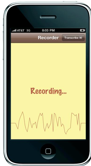
Figure 1: The AudioWiz recording interface running on an iPhone 3GS. Across the lower portion of the screen scrolls a constantly updating visualization of the current thirty seconds of audio available for transcription.
