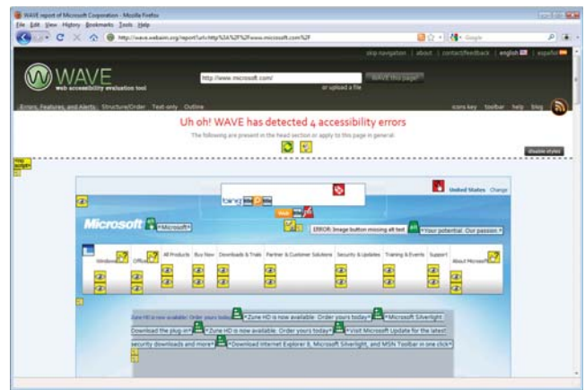
Figure 2: The WAVE accessibility evaluation tool’s analysis of a web page showing numerous warnings, many of which are not actually problems.
