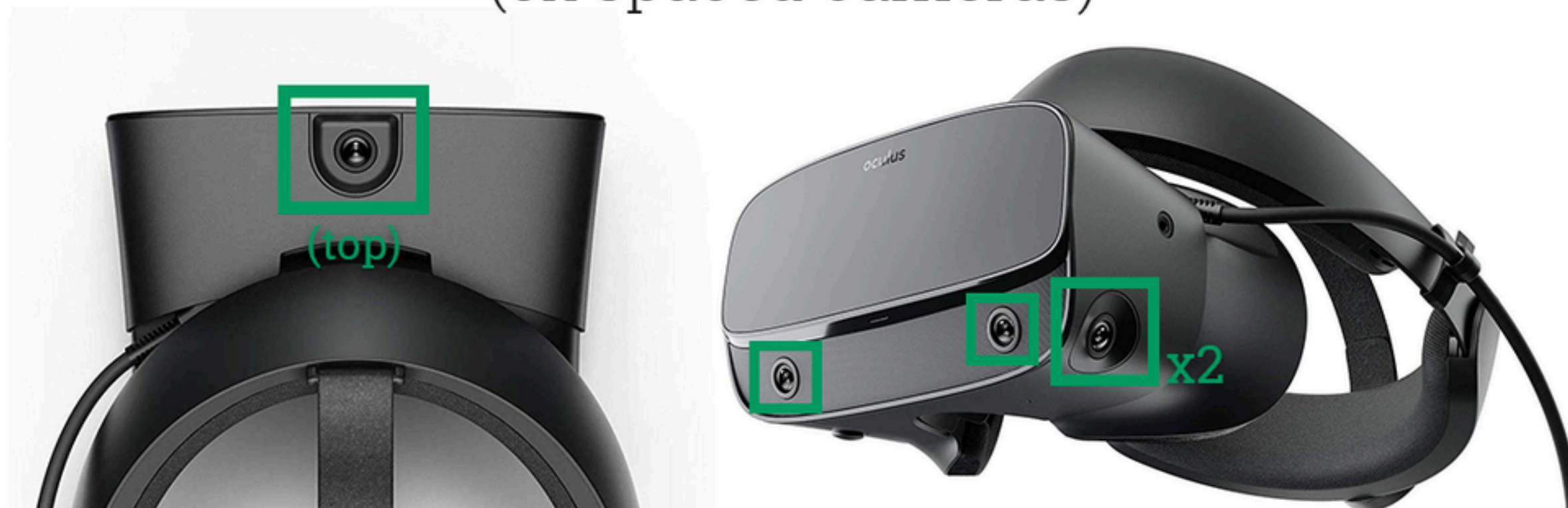
Oculus Rift S (5x spaced cameras)
