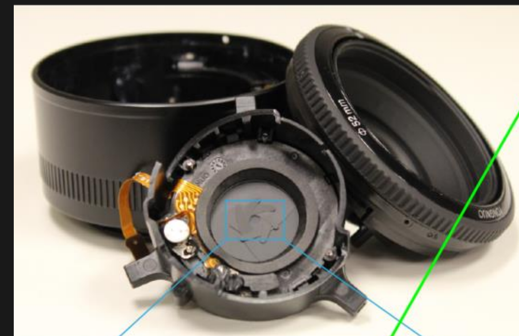
Fabricated phase mask
