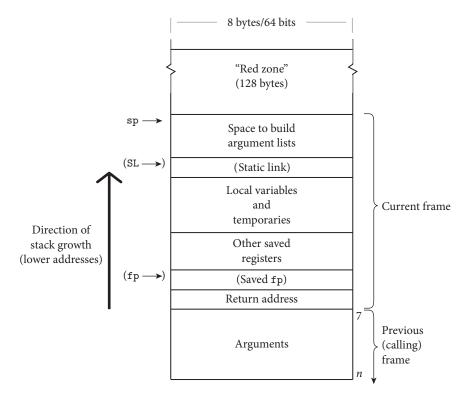
**Figure 9.10** Layout of the subroutine call stack for the GNU Compiler Collection (gcc) on 64-bit x86. Conventions differ from those of Figure C-9.9 in three principal ways: (1) most data are 64 bits wide; (2) the first 6 integer arguments are passed in registers rather than on the stack; (3) leaf routines are permitted to use up to 128 bytes of space beyond the top of the stack, without updating the sp.
