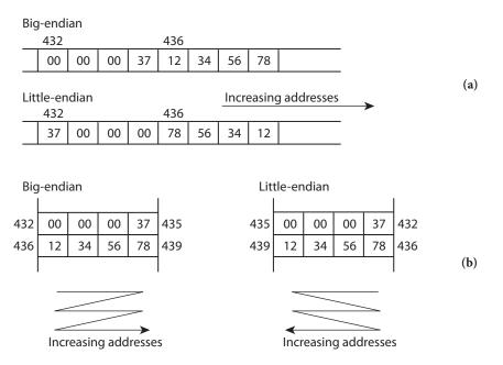
**Figure 5.2** Big-endian and little-endian byte orderings. (a) Two 4-byte quantities, the numbers  $37_{16}$  and  $12\,34\,56\,78_{16}$ , stored at addresses 432 and 436, respectively. (b) The same situation, with memory visualized as a byte-addressable array of words.
