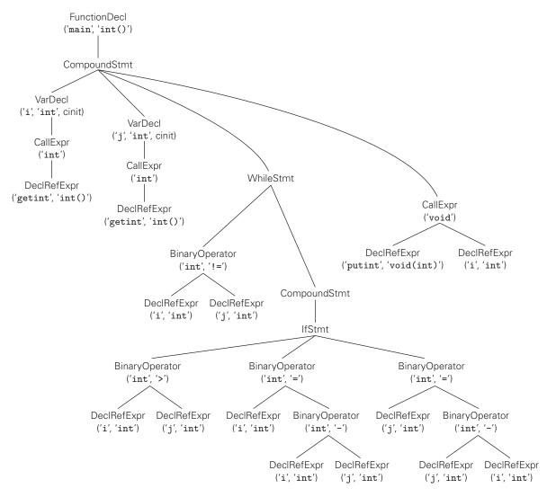
**Figure 15.13** Simplified clang AST for the gcd program. Nodes that implicitly dereference variables (Ivalues) to obtain their contents (rvalues) have been elided.
