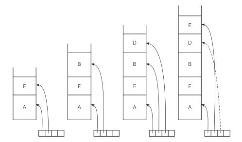
**Figure 9.7** Nonlocal access using a display. The stack configurations, from left to right, illustrate the contents of the display (at bottom) for a sequence of subroutine calls, assuming the lexical nesting of Figure 9.1. Display elements beyond that of the currently executing subroutine are not used.
