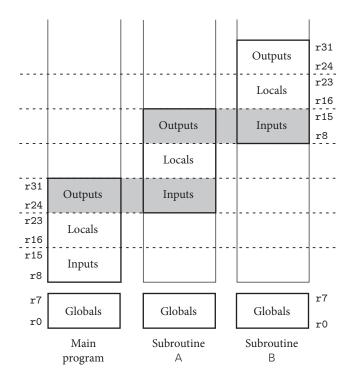
**Figure 9.11** Register windows. When the main program calls subroutine A, and again when A calls B, register names r0-r7 continue to refer to the same locations, but register names r8-r31 are changed to refer to a new, overlapping window. High-numbered registers in the caller share locations with low-numbered registers in the callee.
