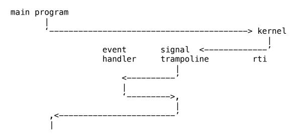
Note that because the main program and signal handler run on the same thread, they can't use scheduler-based locks to synchronize access to shared data structures. Rather (as we saw in the implementation of thread scheduling in Chap. 13), the main program needs to turn off signals while manipulating data that may also be accessed in a handler.
