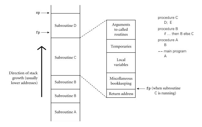
Local variables and arguments are assigned fixed *offsets* from the stack pointer or frame pointer at compile time
