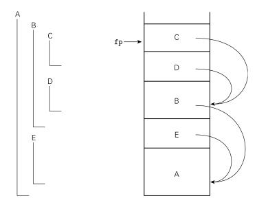
You access a variable in a scope k levels out by following k static links and then using the known offset within the frame thus found.
