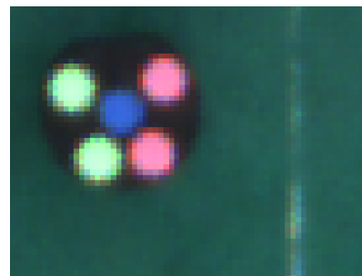
Fig 1: The image acquired from a robot and a white band on a green carpet. The Color artifacts are a result of naïve demosaicing process, not physical phenomena such as a surface reflection.
