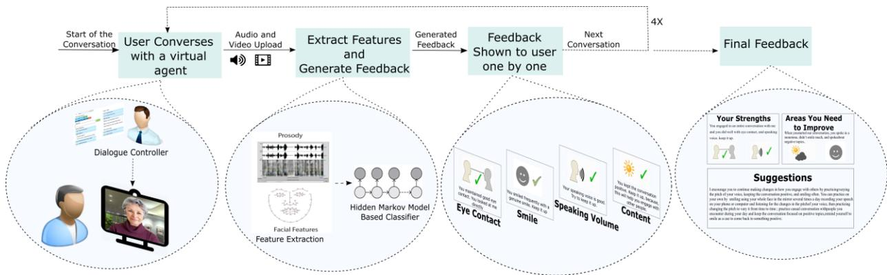
**Figure 2. The overall system. Users initiate a conversation, which is driven by a dialogue controller. Conversation audio and video are processed in the server and feedback are generated. Users receive the feedback one by one and move to the next conversation phase. After four rounds of conversation, users receive final feedback summarizing the previous feedback.**
